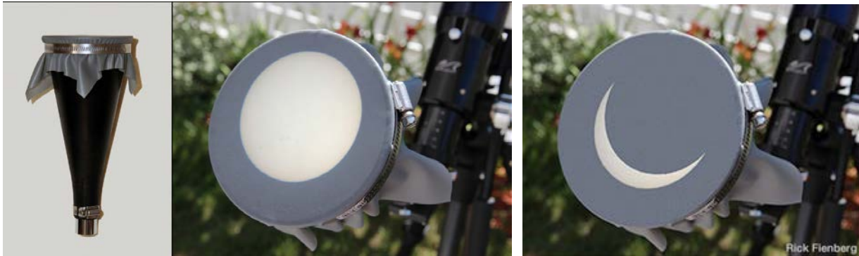
Observing an eclipse with a Sun funnel
